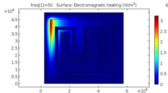
Fig 6: Electromagnetic heating inside micro-transformer due to electric and magnetic field.
