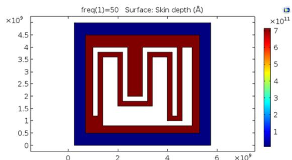
Fig 7: Skin depth inside micro-transformer due to electric and magnetic field.
