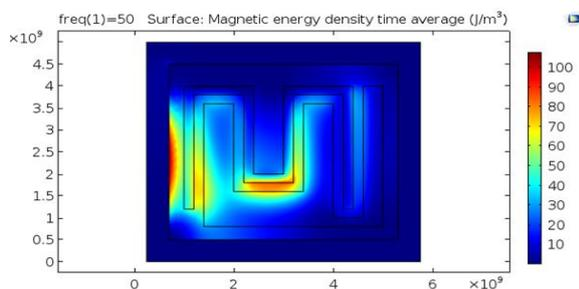
Fig 4: Magnetic energy density obtained after simulating the micro-transformer.
