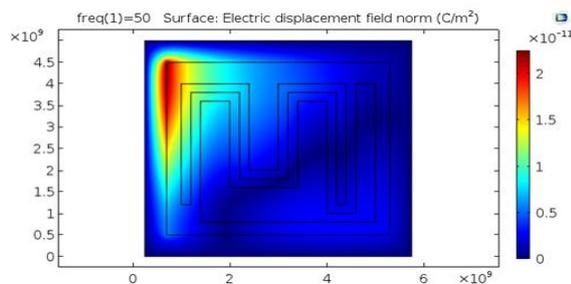
Fig 3: Electrical displacement obtained after simulating the micro-transformer.
