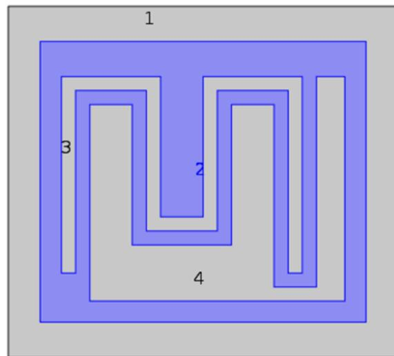
Fig 1: 2D schematic layout of the micro-transformer.
